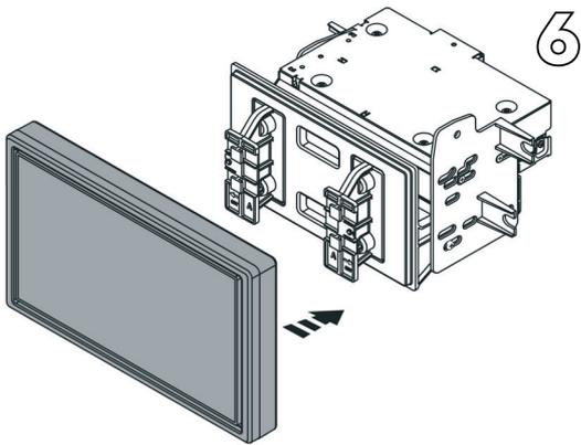
Plug the RGB display cable into the display, then slide and lock in place the display housing to the display brackets. **Note:** The locking pins can be pulled back to release the display housing.
