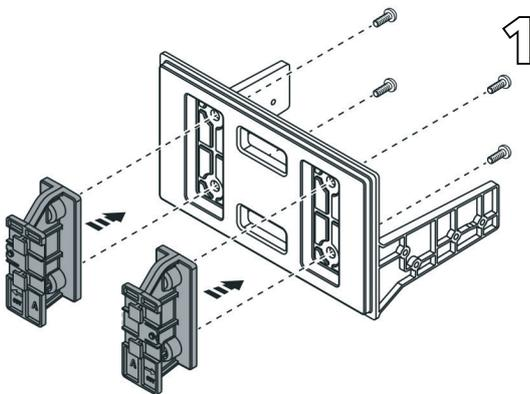
Secure the display brackets to the assembly mount using (4) Allen head screws provided. **Note:** The brackets have a locking pin on them which must face outwards.
