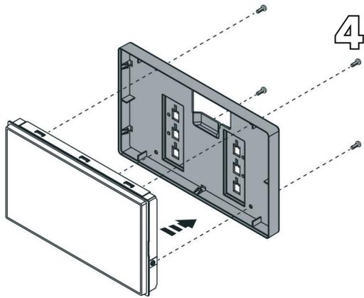
Secure the radio display to the display housing using (4) screws supplied with the radio.
