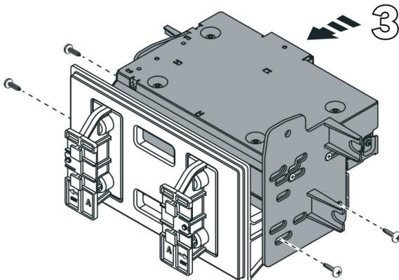
Secure the assembly mount to the brackets of your 2-DIN kit using (4) Phillips screws provided. Route the RGB display cable from the radio chassis, through the opening in the assembly mount.
